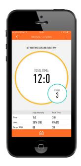
To change the number of cycles tap on the cycles circle. Scroll through to your desired number. Click anywhere else on the screen to exit this setting. As you change the number of cycles the total time will also change in correspondence.
