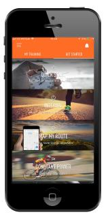
Once you have clicked on the 'Interval' button you will then need to connect your device to the machine you are working out on. Also, select your heart rate source at the bottom of the screen. Once your machine has been connected the monitor will power off and your device will now display the data.
